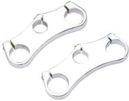
MODEL: JDF05 P C D: 132mm side bore: \phi 38 mid bore(up): \phi 25.5/ \phi 28.7 mid bore(down): \phi 26.97/ \phi 29.97
