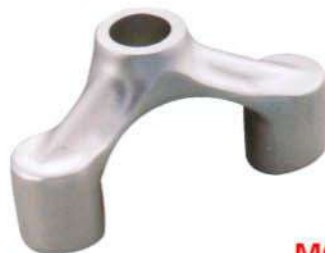
MODEL: JSF11 P C D: 120mm mid bore: \phi 29.97/ \phi 26.97 side bore: \phi 25.20/ \phi 28.45
